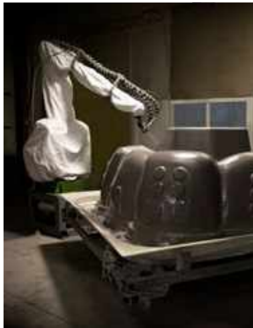
21 ST CENTURY TECHNOLOGY POLI-MAX POLYURETHANE ACRYLIC REINFORCEMENT APPLIED BY ABB ROBOT
