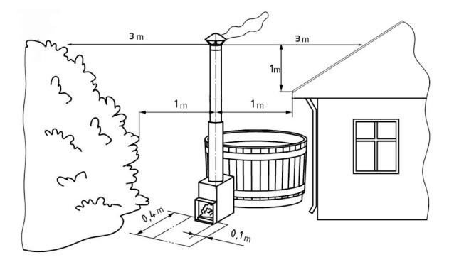
When placing the hot tub near buildings, the distance between the fireplace pipe and combustible structures must be at least that shown in the sketch. Remember to check the distance both sideways and vertically. It is important to prevent the risk of ignition. Local regulations may vary.
